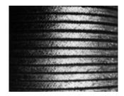
4062AF is manufactured from the highest grade carbon yarn with an Inconel Wire carrier. This proven material is braided over a core of graphite and exclusive corrosion inhibitors which prevent stem pitting. 4062AF non-hardening valve stem packing, will also provide many years of service in expansion joints. Temp.: To 1200°F (649°C). Pressures: To 1200 psi and beyond.
