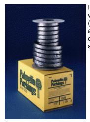
Interwoven<sup>™</sup> braid of carbon fiber, Palcar<sup>™</sup> is impregnated with graphite particles, which makes it ideal for boiler feed pumps, blowers, and driers. Temp. 1200°F (650°C) in steam, 650°F (345°C) in oxygen and 2400°F (1320°C) in reducing atmosphere. pH 1-14. Style 1585 exhibits extremely low coefficient of friction characteristics enabling dynamic equipment ease of operation and long trouble-free service life.
