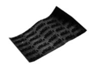
2970 is the direct replacement for asbestos sheet gasketing. Manufactured of predominantly Aramid Filament with premium NBR binders assures long shell life vs. asbestos sheet. Style 2970 is soft and compressible and is highly recommended for such applications as pipe flanges, mixers, ovens, kettle, manifolds, digesters, tanks, columns and pumps. Temp. 750°F (399°C). Leachable Chloride content is less than 100 ppm which helps prevent flange pilling.
